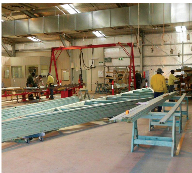
Roof truss manufacturing
